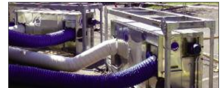
Wet side, MS-6000/5000 pulls moisture from ambient air.
